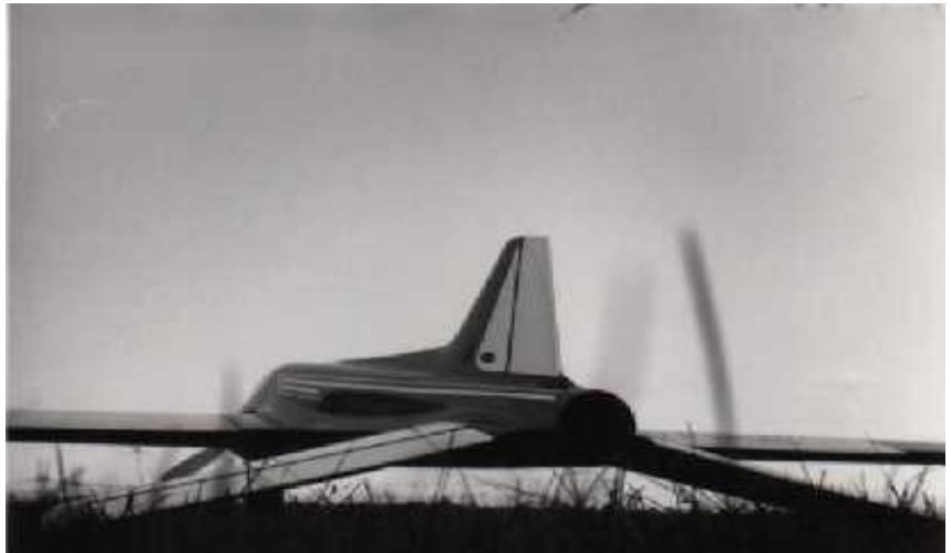
Dawn Patrol. Single retract nosewheel with wheels in the tailplane tips left the underside of the wing perfectly clean. No disturbed air from wheel wells. A very fast aerobatic model.
