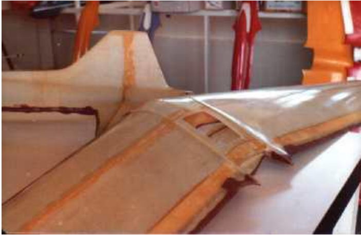
Stingray components straight out of the mould. Glasswork by Alan Trinder, aircraft design by Bob Young. Model came out of the moulds in two pieces. Joined fuselage with integral fin and tailplane and complete wing.
