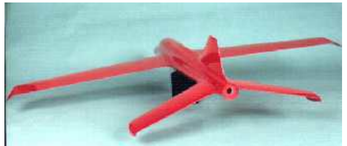
Wooden plug for Silvertone Stingray-A one of the world's first all fibreglass models. (c1974)
