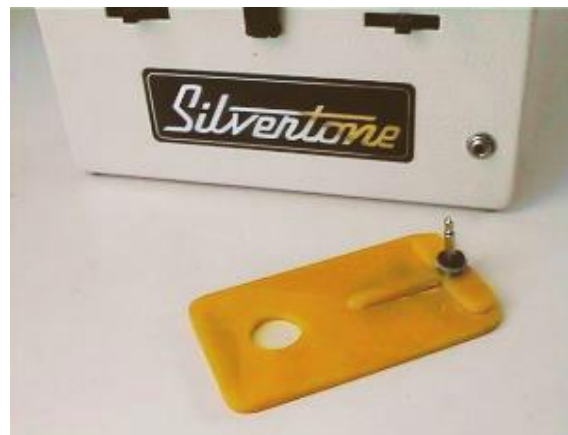
Reverse side of key showing Interlock plug. Key plugs into TX when not in use cutting off all power to the transmitter, thus rendering it safe when returned to the pits.
