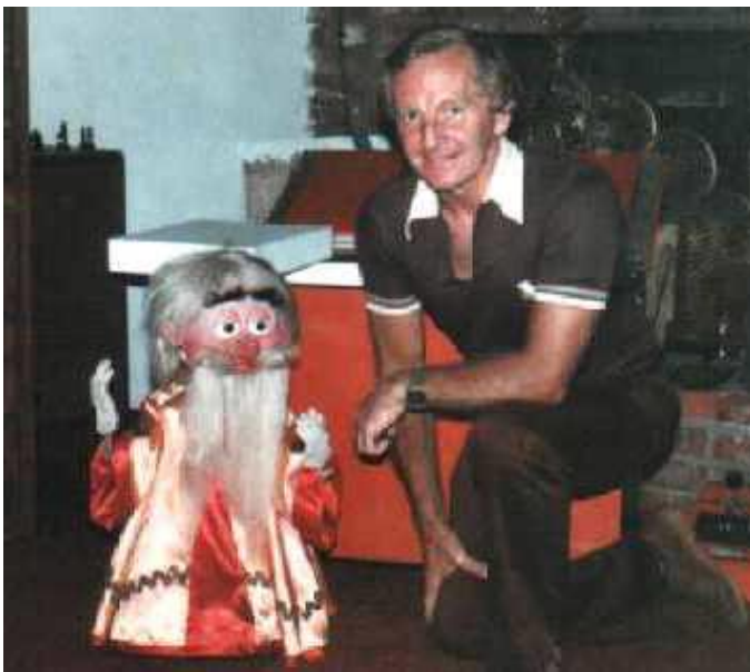
Bob Young with Alakazam the Robotic Puppet (Dummy on the left). Thirty-two channels, voice synchronous lips, blinking eyelids. Control tape was built up in layers, four channels at a time. All before computers. Used in a Hollywood Children's TV pilot trilogy.
