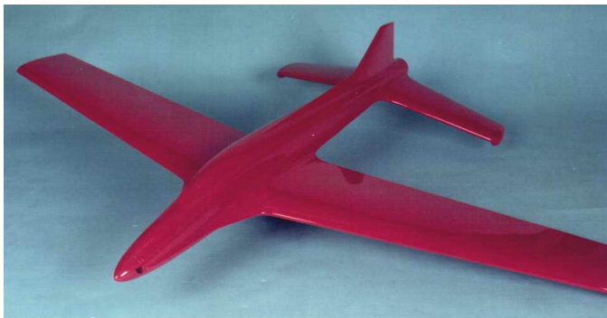
Wooden plug for Silvertone Stingray-A one of the world's first all fibreglass models. (c1974)
