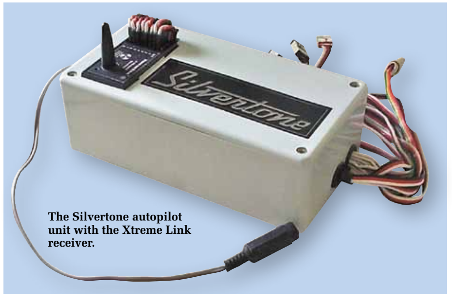
This view shows the Xtreme Link receiver installed in an autopilot housing. Note the tidy lead arrangement.
