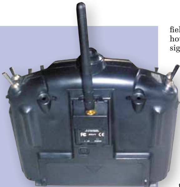
The Futaba 9C transmitter with the Xtreme Link 2.4GHz DSSS module in place of the 36MHz module. Note the small rubber duck antenna.
